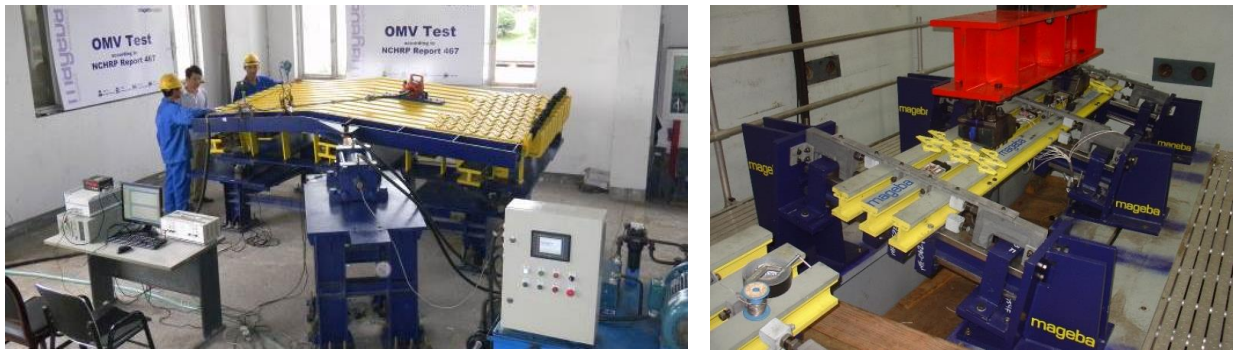
Figure 1: On left, Opening Movement and Vibration [OMV] test; on right, fatigue testing – one of the ten required test specimens, each subjected to six million load cycles
